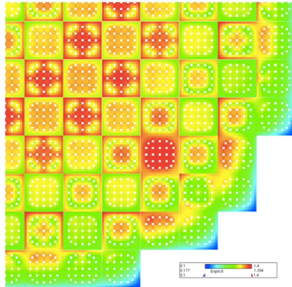
Figure 17. MC21 pin wise relative power density at day 92.
