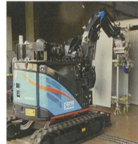
Remote-controlled heavy machinery (ASTACO-SoRa)
